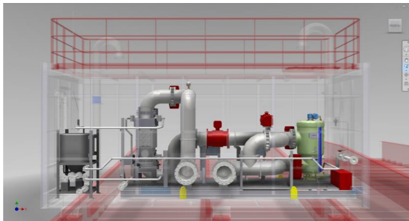
Photo top left Detail of piping and mechanical package designed to treat a maximum flow of 1.500 m 3 /h.
